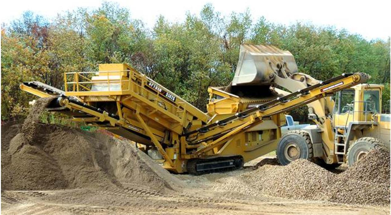
Screen Machine Industries LLC is proud to announce the newest addition to their extensive product line, the Spyder 514TS. This unit is a patented, track-mounted reverse style screening plant designed for secondary screening of rock, sand & gravel, and other materials. Equipped with a 5'x14' double-deck screen with *Smooth Start® Technology*, this heavy-duty machine is capable of producing up to three different finished sized products simultaneously.
