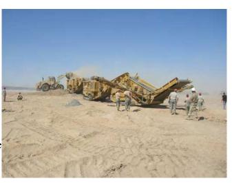
and ¾" wire mesh bottom deck screens. This allowed the Airmen to generate two separate usable products while also sorting out the trash. The fine material would be mixed back into new concrete mixes while the mid sized product could be used for road base.
