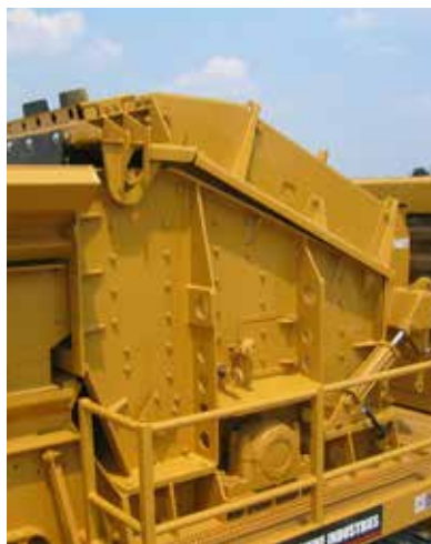
Crusher chamber with its lid lifted via the Crusher Relief System™
