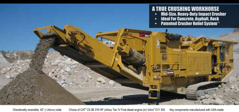
conveyor with impact bed and guide idlers creates maintenance-free material flows
