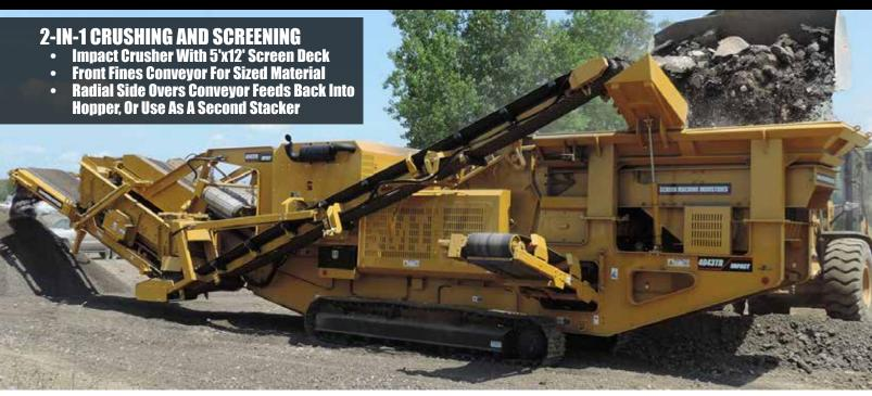
48" (1,219mm) wide fines conveyor delivers sized material off the front of the machine
