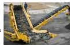
Fines Belt Discharge Height 12'- 6" (3.8m) Midsize Belt Discharge Height 13' - 0" (3.8M) Oversize Belt Discharge Height 9' - 6" (2.9m)
