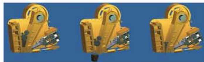
Blockage Clearance (JXT)
