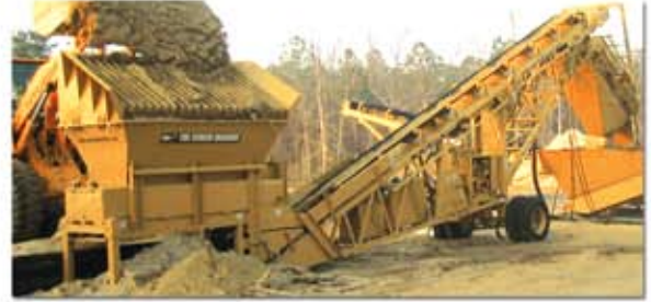
Producer with 4"x8" (1.2m x 2.4m) double deck wash arrangement with 36" (.91m) screw and two 40' (12.2m) stacking conveyors
